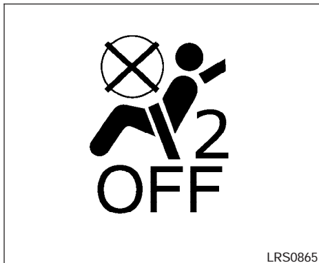
Front passenger air bag and status light
