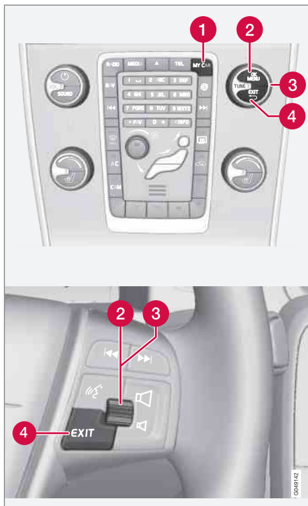
Control panel in centre console and steering wheel keypad. The figure is schematic - the number of functions and layout of the buttons both
