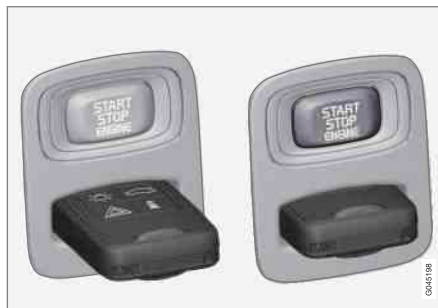
Ignition switch with remote control key extracted/inserted.
