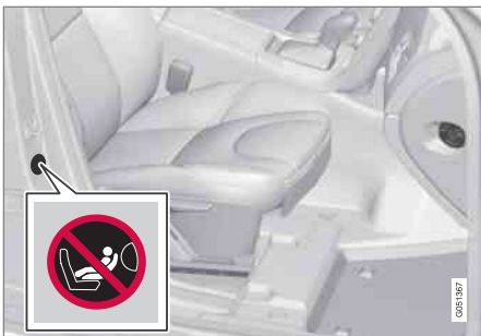
Alternative 2: Position of airbag label on passenger side door pillar. The label becomes visible when the passenger door is opened.
