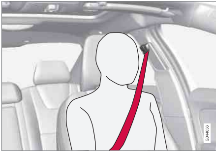
Correctly fitted seatbelt.
