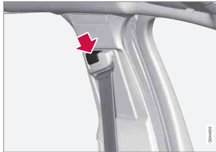
Seatbelt height adjustment. Press the button and move the belt vertically. Position the belt as high as possible without it chafing against your throat.
