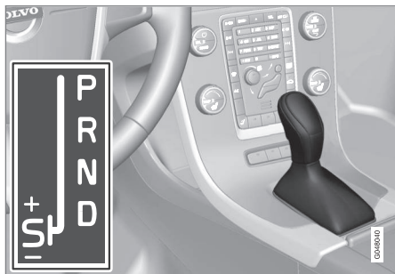
D: Automatic gear positions. +S- : Manual gear positions. S: Sport mode*.
