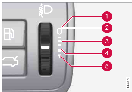
Thumbwheel positions for different load cases.
