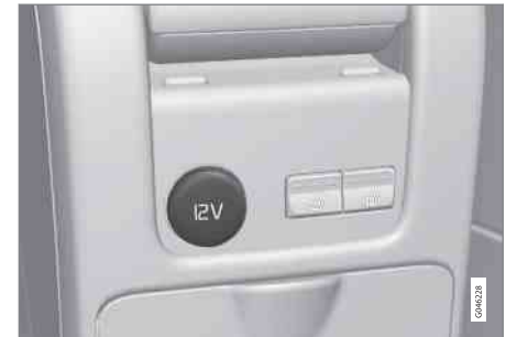
12 V socket in tunnel console, rear seat.
