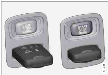
Ignition switch with remote control key extracted/inserted.
