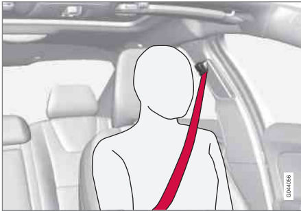
Correctly fitted seatbelt.
