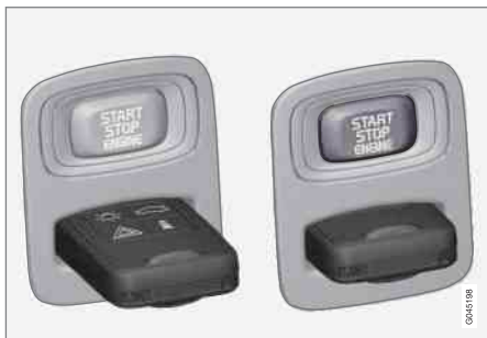
Ignition switch with remote control key extracted/inserted.
