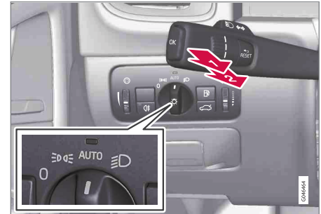
Stalk switch and knob for headlamp control.
