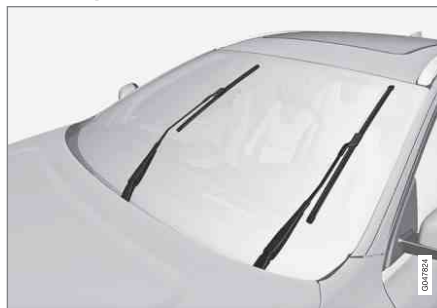
Wiper blades in service position.
