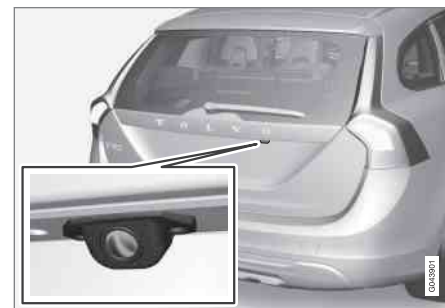
Camera location next to the opening handle.
