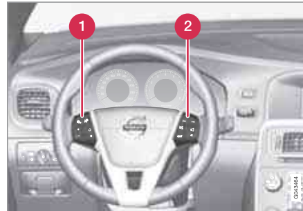
Keypads in the steering wheel.
