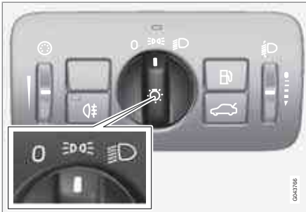
Headlamp control in position for position/parking lamps.
