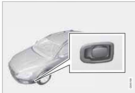
Electrical input to the engine block heater.
