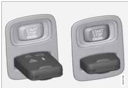
Ignition switch with remote control key extracted/inserted.
