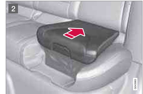
2 Press the booster cushion backwards to lock.
