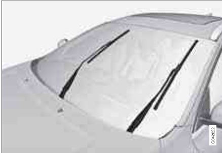
Wiper blades in service position.
