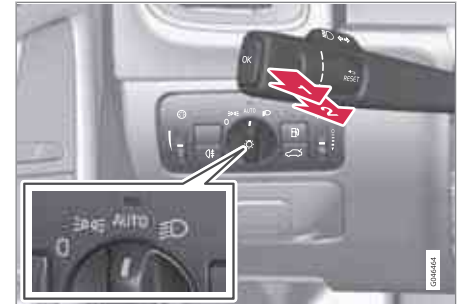
Headlamp control and stalk switch.
