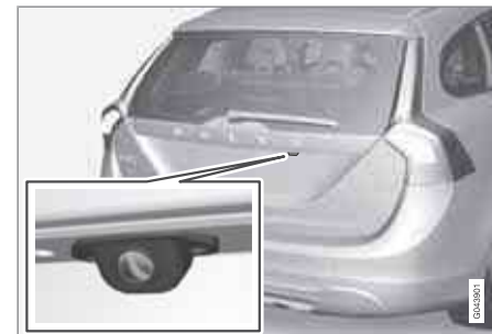
Camera location next to the opening handle.
