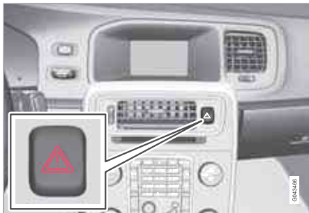
Button for hazard warning flashers.
