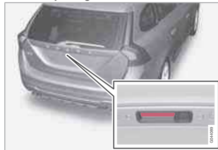
Rubber plate with electrical contact.
