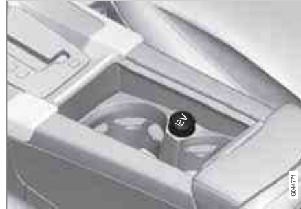
12 V socket in tunnel console, front seat.
