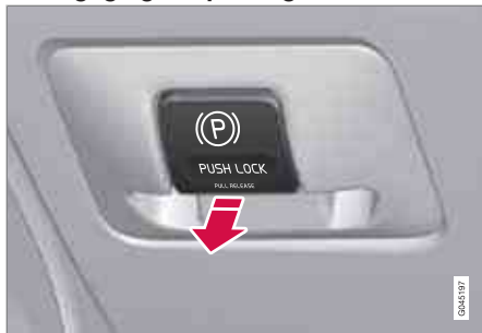
Parking brake control - release.
