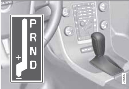
D: Automatic gear positions. +/-: Manual gear positions.
