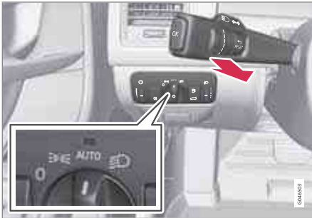
Headlamp control and stalk switch.
