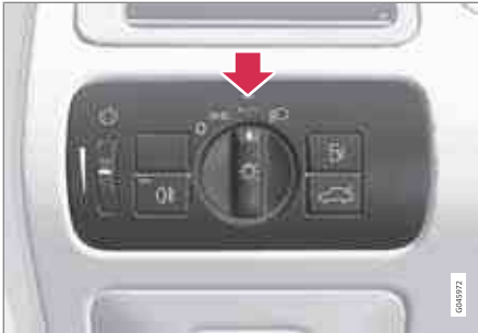
Light switch in position AUTO .
