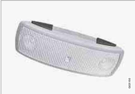
Rear roof lighting.
