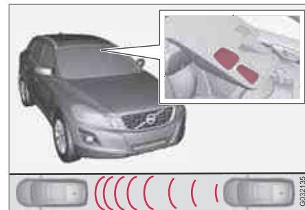
Laser sensor transmitter and receiver window 1 .
