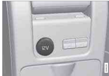
12 V socket in tunnel console, rear seat.
