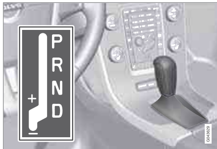
D: Automatic gear positions. +/-: Manual gear positions.
