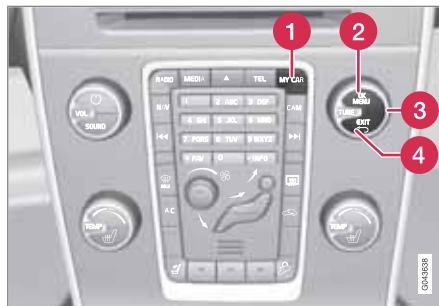
Centre console controls for menu navigation.
