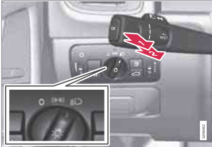
Headlamp control and stalk switch.
