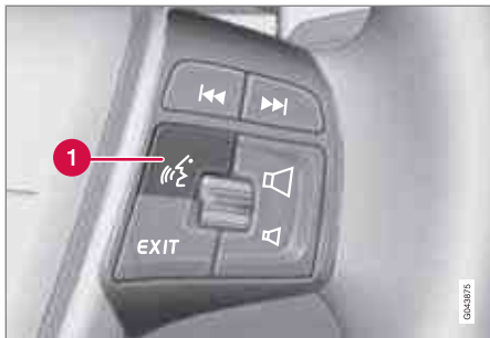
Steering wheel keypad.
