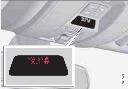
Seat belt reminder light in ceiling console
