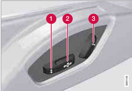
Power seat adjustment controls
