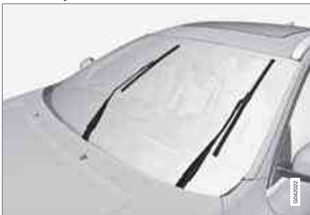
Wiper blades in service position
