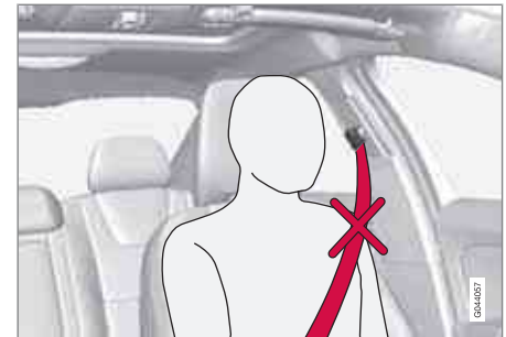
Incorrect height adjustment
