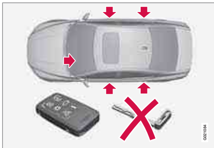
Locking/unlocking points with valet locking activated
