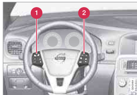
Keypads in the steering wheel
