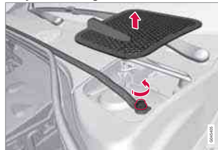
Rally bar and bulkhead hatch
