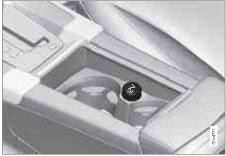
12-volt socket in the front tunnel console
