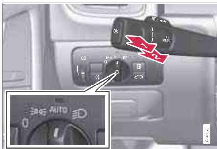
Headlight switch with AUTO and lever
