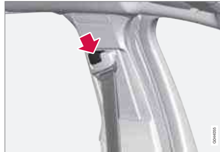
Adjusting seat belt height
