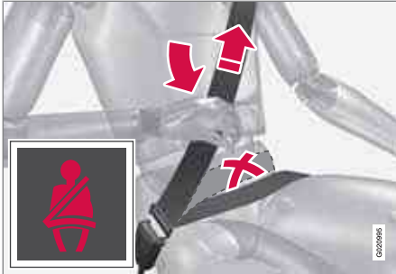
Adjusting the seat belt
