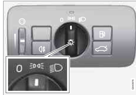
Headlight control in position for parking lights
