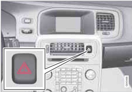
Location of the hazard warning flasher button
