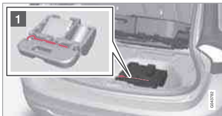
Location of the towing eyelet
