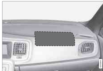
Location of the passenger's side front airbag
