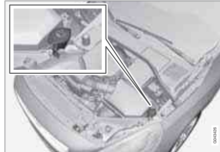
Location of the washer fluid reservoir
