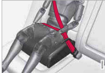
Positioning the seat belt
