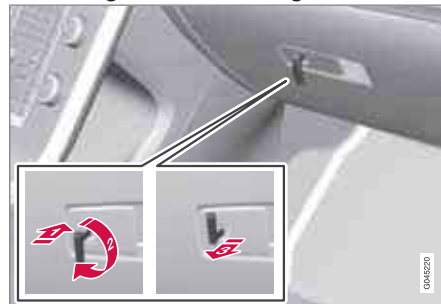
Locking/unlocking points with valet locking activated
