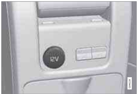
12-volt socket in the rear center console
