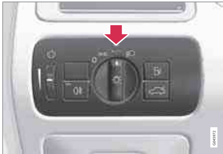
Light switch in the AUTO position
