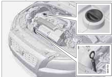
Location of the filler cap and dipstick
