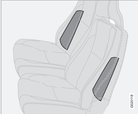
Location of the side impact (SIPS) airbag
