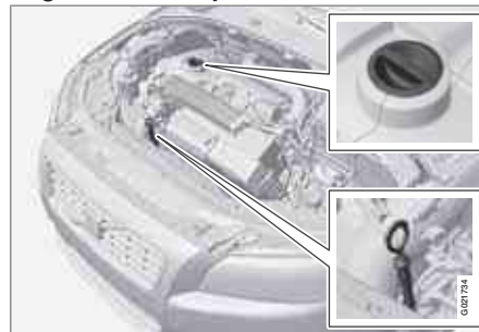
Dipstick and filler pipe.
