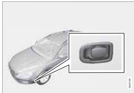
Electrical input to the engine block heater.
