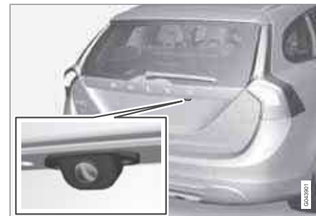
Camera location next to the opening handle.
