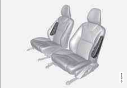
Location of the side impact (SIPS) airbags (front seats only)
