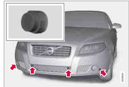
Location of the front sensors
