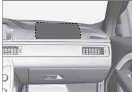
Location of the passenger's side front airbag
