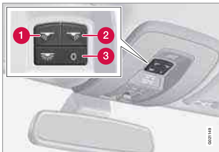
Light switches, front roof lighting
