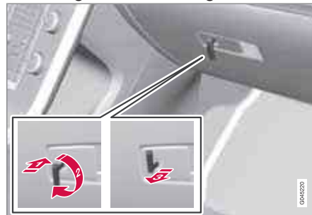
Locking/unlocking points with valet locking activated
