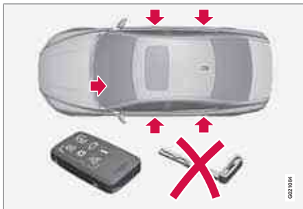
Locking/unlocking points with valet locking activated
