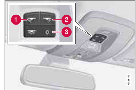
Light switches, front roof lighting
