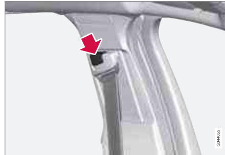
Adjusting seat belt height
