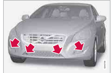
Location of the front sensors
