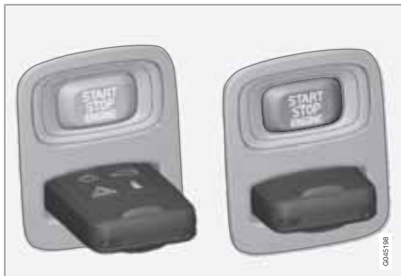
Ignition switch with remote key inserted ( see page 86 for more information on ignition modes)
