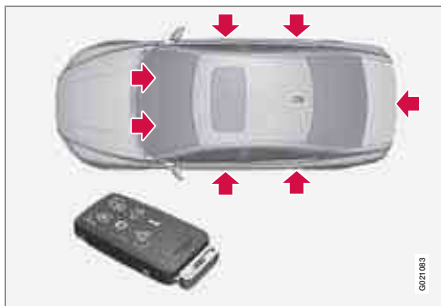
Normal locking/unlocking function
