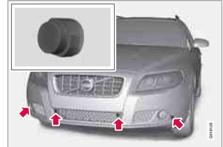
Location of the front sensors
