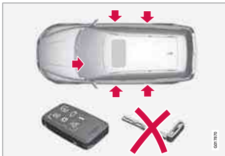
Locking/unlocking points with private locking activated.
