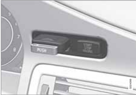
Ignition switch with remote key inserted (see page 79 for more information on ignition modes)
