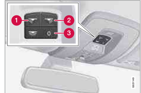
Light switches, front roof lighting
