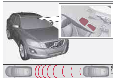
Laser sensor transmitter and receiver window.
