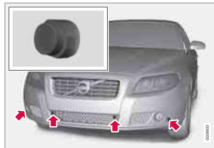
Location of the front sensors
