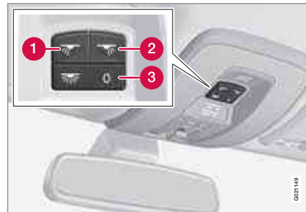
Light switches, front roof lighting
