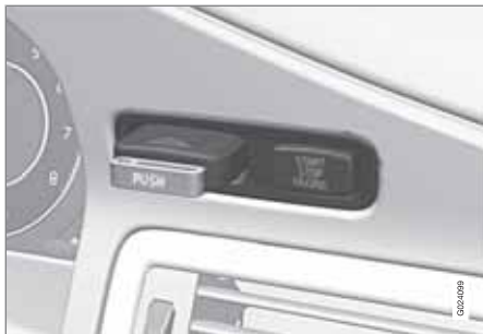
Ignition switch with remote key inserted (see page 78 for more information on ignition modes)
