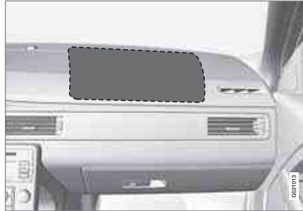
Location of the passenger's side front airbag
