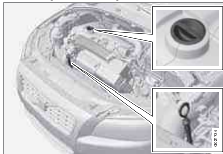
Location of the filler cap and dipstick
