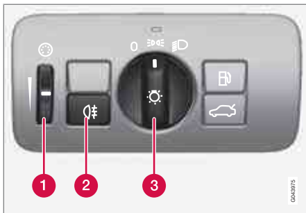
Overview, light switches
