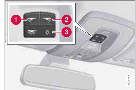
Light switches, front roof lighting
