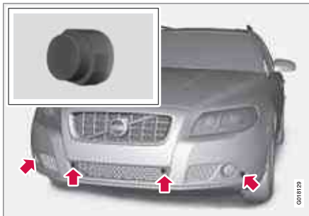
Location of the front sensors.
