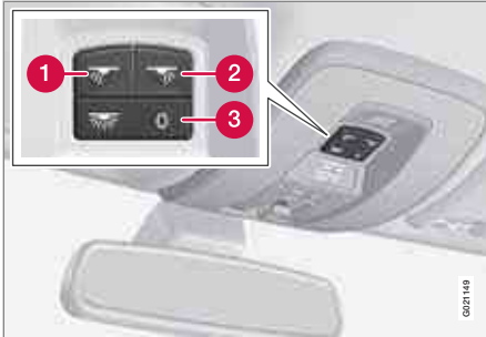
Light switches, front roof lighting
