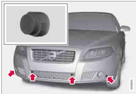
Location of the front sensors.
