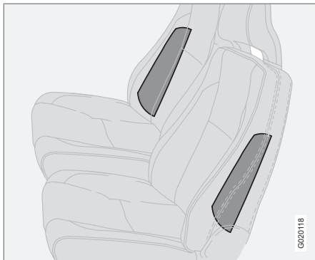
Location of the side impact (SIPS) airbag
