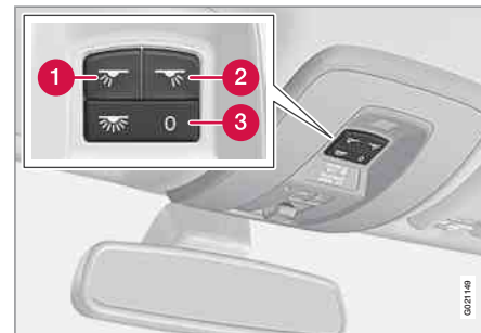
Light switches, front roof lighting
