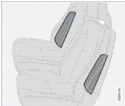
Location of the side impact (SIPS) airbag
