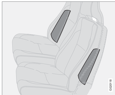
Location of the side impact (SIPS) airbag
