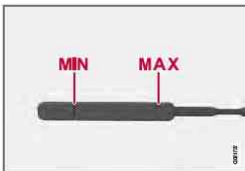
The oil level must be between the MIN and MAX marks on the dipstick
