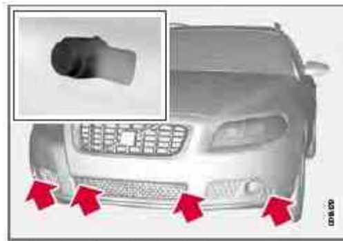
Location of the front sensors
