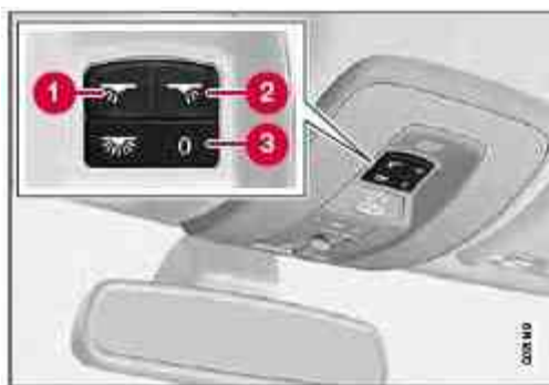
Light switches, front roof lighting
