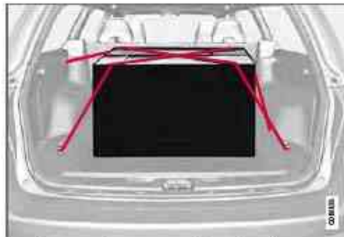
Load secured in upper and lower hooks
