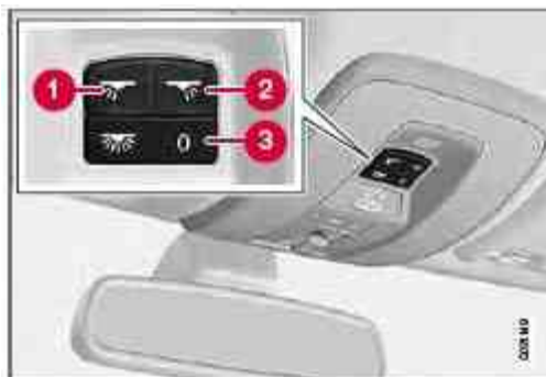
Light switches, front roof lighting
