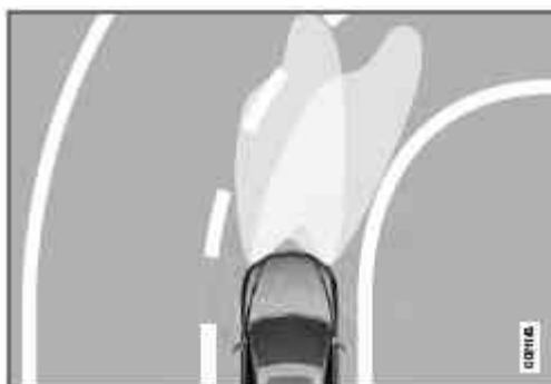
Headlight pattern with ABL deactivated (left) and activated (right) respectively
