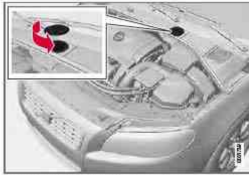
Location of the brake fluid reservoir
