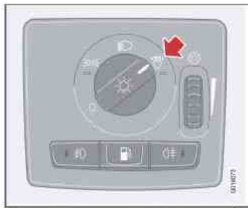
Lighting panel, vehicles with Active Bi-Xenon® headlights
