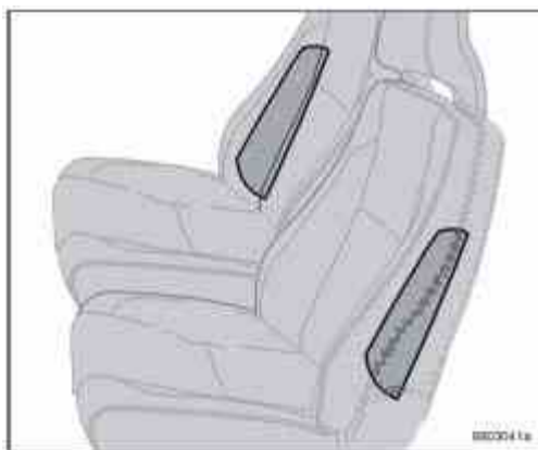
Location of the side impact (SIPS) airbag
