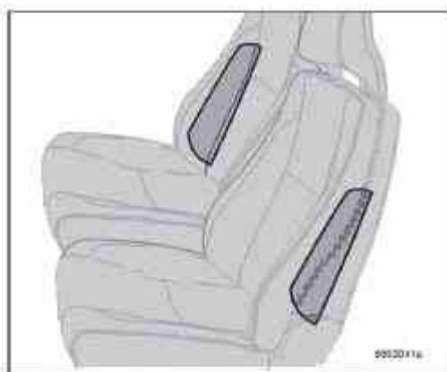
Location of the side impact (SIPS) airbag
