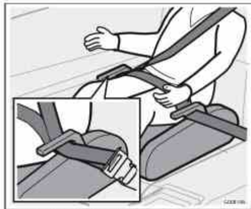
Position the child correctly on the booster cushion and fasten the seat belt.
