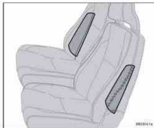
Location of the side impact (SIPS) airbag
