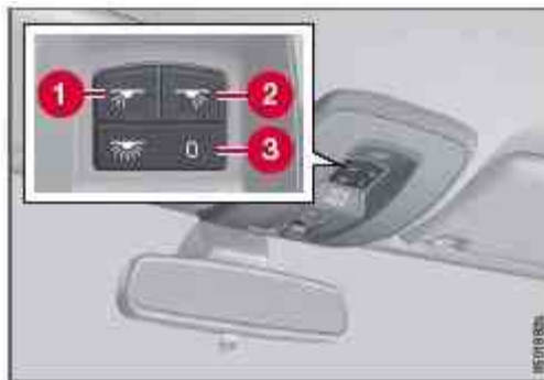
Light switches, front roof lighting
