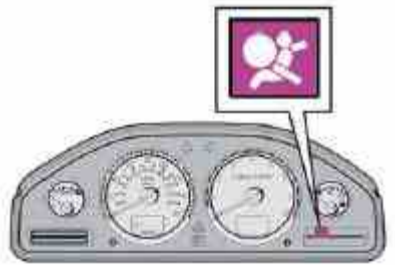
SRS warning light
