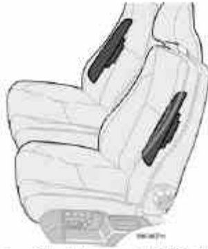
Location of the side impact (SIPS) airbag
