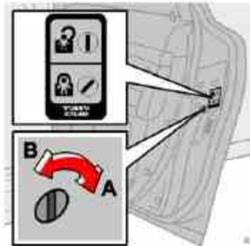
Control for child safety lock - right rear door
