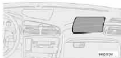
Passenger's side airbag—above glove compartment
