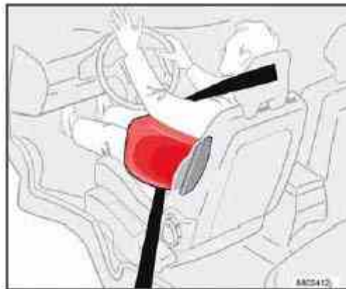
Components in the SIPS airbag system
