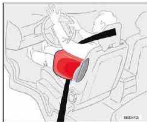
Components in the SIPS airbag system
