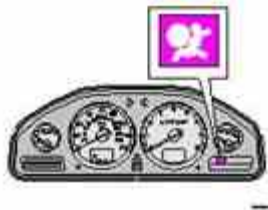
SRS warning light
