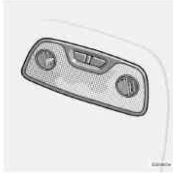
Rear reading lights (in ceiling)
