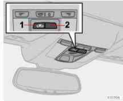
1. Disabling the double locking feature and the accessory alarm sensors 2. Not in use
