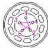
Correct tightening order for wheel bolts
