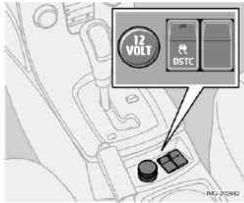
12 volt socket, stability system, auxiliary equipment
