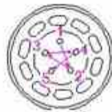
Correct tightening order for wheel bolts
