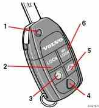
1 - Fold key in/out, 2 - Lock, 3 - Approach lighting, 4 - "Panic" function, 5 - Open trunk, 6 - Unlock
