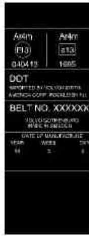
Sample label found on all seat belts with tensioners
