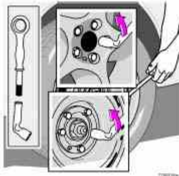
Loosen the wheel bolts
