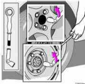
Loosen the wheel bolts
