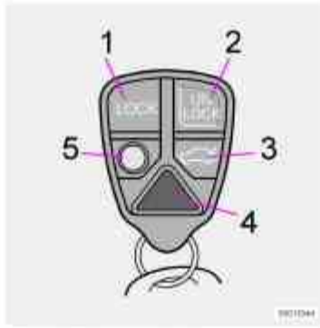
Buttons in remote control: 1 - Lock, 2 - Unlock, 3 - Open trunk, 4 - "Panic" function*, 5 - Approach lighting
