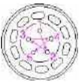
Correct tightening order for wheel bolts
