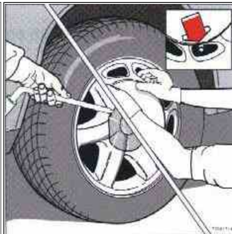
Insert flat end of lug wrench and turn Pull straight out
