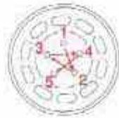
Correct tightening order for wheel bolts
