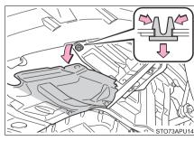
3 Partly remove the fender liner.
