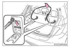
5 Lay the flat tire on the luggage floor so that the outer side of the tire wheel faces toward the rear of the vehicle. Detach the rear center head restraint from the seat and release the belt.
