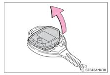
Open the battery cover using a coin protected with tape etc., and remove the depleted battery.
