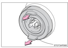
Release the bulb retaining spring.
