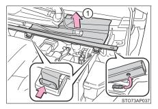
2 Remove the battery terminal cover and then the fuse box cover.
