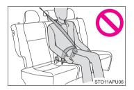
Do not allow anyone sit on the rear center seat if the rear right seat is folded down, as the seat belt buckle for the rear center seat belt is then concealed under the folded seat and cannot be used.
