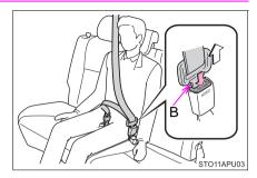
2 To release the hooked plate "A", insert the plate "B", the key into the hole on the buckle.
