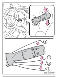
Washer/wiper dual operation The wiper will automatically operate a couple of times after the washer squirts.
