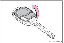
3 Open the case cover and remove the depleted battery.
