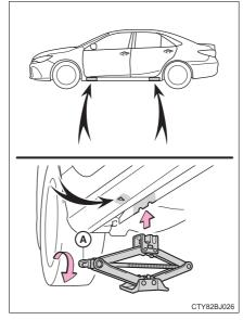
5 Raise the vehicle until the tire is slightly raised off the ground.
