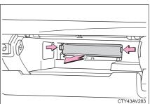
4 Remove the air conditioning filter and replace it with a new one.
