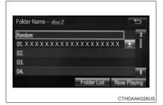
When an MP3/WMA/AAC disc or USB memory device is being used, the folder can be selected. When a Bluetooth  $^{\tiny (\!R\!)}$  device or iPod is being used, the album can be selected.
