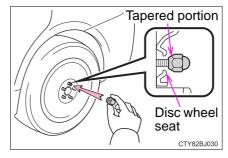
When replacing an aluminum wheel with a steel wheel, tighten the wheel nuts until the tapered portion comes into loose contact with the disc wheel seat.
