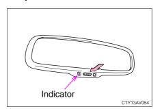
Vehicles with a smart key system: The function will set to ON mode each time the engine switch is turned to IGNITION ON mode.
