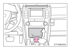
Open the cover and connect an iPod using an iPod cable. Turn on the power of the iPod if it is not turned on.
