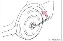
4 Turn the tire jack portion "A" by hand until the notch of the jack is in contact with the jack point.
