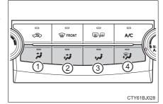
(4) Air flows to the feet and the windshield defogger operates.
