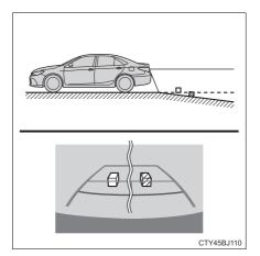
When any part of the vehicle sags due to the number of passengers or the distribution of the load, there is a margin of error between the fixed guide lines on the screen and the actual distance/course on the road.
