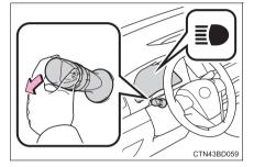
2 Press the Automatic High Beam switch.
