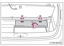
4 Remove the jack after removing the hook.
