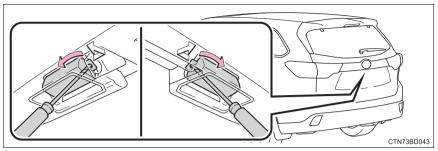
Insert a properly sized screwdriver into the hole of the lens on the inner side and disengage the claw and pry the lens toward the outer side as shown in the illustration.
