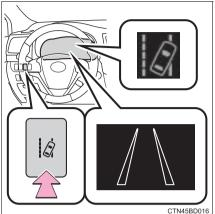
Press the LDA switch to activate the system.
