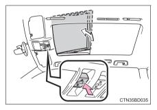
The moon roof can be tilted down only when it is in the tilt-up position.
