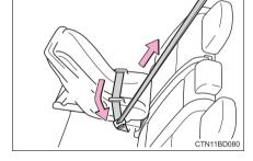
After the shoulder belt has retracted to a point where there is no slack in the belt, pull the belt to check that it cannot be extended.
