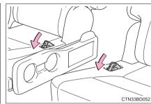
4 Pass the outer seat belts through the seat belt hangers and secure the seat belt plates.
