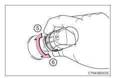
Washer/wiper dual operation Wipers will automatically operate a couple of times after the washer squirts.
