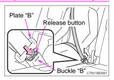
2 To release plate "A", insert the key (→P. 114) or plate "B" into the hole on buckle "A".
