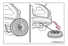
When stowing the tire, make sure that the hoist assembly is placed perpendicular to the wheel opening.
