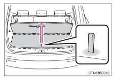
2 To secure the center deck board, remove the hook on the backside of the center deck board and attach the hook to the head restraint on the third seats as shown.
