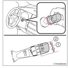
Washer/wiper dual operation The wiper will automatically operate a couple of times after the washer squirts.
