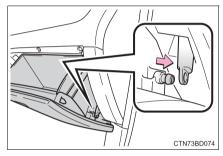
23 Push in the glove box on the vehicle's outer side to disconnect the claws. Then pull out the glove box and disconnect the lower claws.
