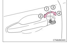
Turning the key rearward unlocks the driver's door. Turning the key once again within 5 seconds unlocks the other doors.
