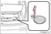
5 Attach the adapter socket to the spare tire clamp bolt.
