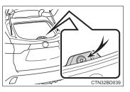
Do not close the glass hatch while the rear wiper is switched on. The rear wiper arm may be restarted suddenly after closing the glass hatch.
