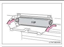
6 Remove the air conditioning filter and replace it with a new one.
