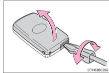
Remove the depleted battery.
