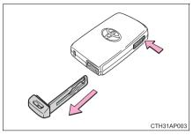
After using the mechanical key, store it in the electronic key. Carry the mechanical key together with the electronic key. If the electronic key battery is depleted or the entry function does not operate properly, you will need the mechanical key. (→P. 618)
