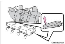
2 Pull the lever to unlock the seatback. The seatback will be folded down.
