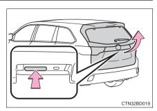
When the back door is locked (vehicles with a smart key system): While carrying the electronic key on your person, press and hold the back door opener switch.
