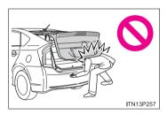
The back door may fall if it is not opened fully. It is more difficult to open or close the back door on an incline than on a level surface, so beware of the back door unexpectedly opening or closing by itself. Make sure that the back door is fully open and secure before using the luggage compartment.
