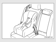
Seat belts equipped with a child restraint locking mechanism (ALR/ELR belts except driver's seat belt) (→P. 109)
