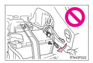
Do not disconnect the negative (-) terminal on the body side as shown. The disconnected negative (-) terminal may touch the positive (+) terminal, which may cause a short and result in death or serious injury.
