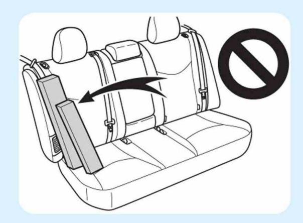
There is an air intake vent on the right side of the rear seatback for the purpose of cooling the hybrid battery (traction battery). If the vent becomes blocked, the hybrid battery (traction battery) may overheat, leading to a reduction in hybrid battery (traction battery) output.
