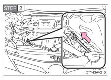
Holding a rag under the end, pull the dipstick out.
