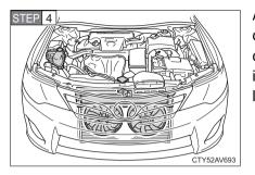
After the hybrid system has cooled down, check the power control unit coolant level and inspect the cooling system for leaks.
