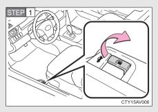
Pull up the opener to open the fuel filler door.
