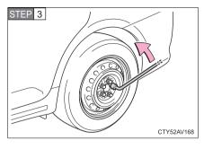
Slightly loosen the wheel nuts (one turn).
