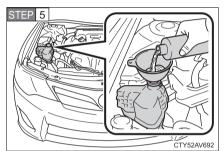
Add power control unit coolant if necessary.
