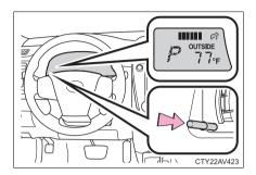
Pressing the button will adjust brightness of the instrument panel lights.
