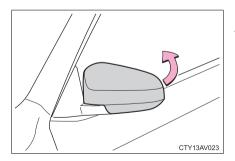
Push the mirror back in the direction of the vehicle's rear.
