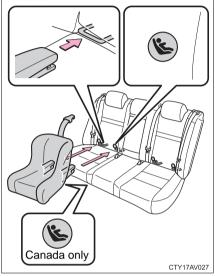
Latch the buckles onto the LATCH anchors. If the child restraint has a top tether strap, the top tether strap should be latched onto the top tether strap anchor.
