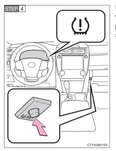
Press and hold the tire pressure warning reset switch until the tire pressure warning light blinks slowly 3 times.
