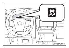
The slip indicator flashes to indicate that the ABS/VSC/TRAC systems are operating.
