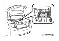
Never try to open the service plug access hole located in the luggage compartment. The service plug is used only when the vehicle is serviced and is subject to high voltage.
