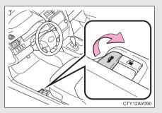
Pull up the lever to release the trunk lid.
