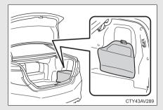
The 12-volt battery is located on the right-hand side of the luggage compartment.
