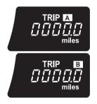
Displays the distance the vehicle has been driven since the meter was last reset. Trip meters A and B can be used to record and display different distances independently.
