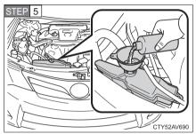
Add engine coolant if necessary.
