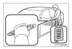
Grip the driver's door handle to unlock the door.\* (Grip the passenger's door handle to unlock all doors.)
