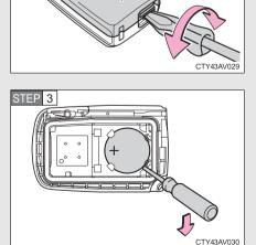
Remove the depleted battery using a small flathead screw-driver.
