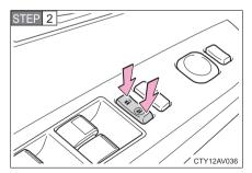
Shift the shift lever to P or N, and press and hold the driver's door lock switch ( or ) for approximately 5 seconds and then release.
