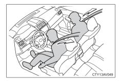
The pretensioner helps the seat belt to quickly restrain the occupant by retracting the seat belt when the vehicle is subjected to certain types of severe frontal or side collision.
