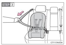
Fully extend the shoulder belt and allow it to retract to put it in lock mode. In lock mode, the belt cannot be extended. Before driving
