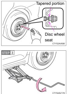
When replacing an aluminum wheel with a steel wheel, tighten the wheel nuts until the tapered portion comes into loose contact with the disc wheel seat.
