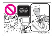
Check that the shift lever is securely set in P. The hybrid system may not start if the shift lever is displaced out of P. "SHIFT TO P POSITION TO START" will be displayed on the multi-information display.
