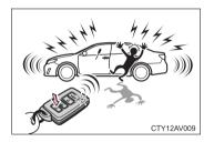
When ((1) is pressed for longer than about one second, an alarm will sound intermittently and the vehicle lights will flash to deter any person from trying to break into or damage your vehicle.
