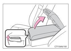
Lift the lid while pulling up the lever to release the lock.
