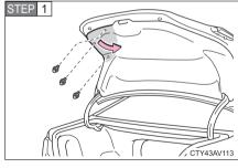
Open the trunk lid and remove the clips. Then partly remove the trunk panel cover.
