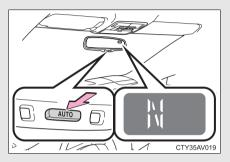
To turn the compass on or off, press "AUTO" for more than 3 seconds.
