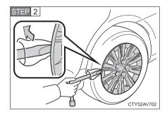
For vehicles with steel wheels, remove the wheel ornament using the wrench.
