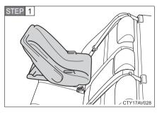
Place the child restraint system on the rear seat facing the rear of the vehicle.
