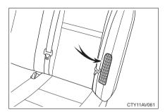
There is an air intake vent beside the rear left seat for the purpose of cooling the hybrid battery (traction battery). If the vent becomes blocked, the hybrid battery may overheat, leading to a reduction in hybrid battery output.
