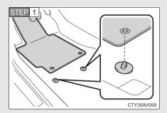
retaining Insert the hooks (clips) into the floor mat evelets.
