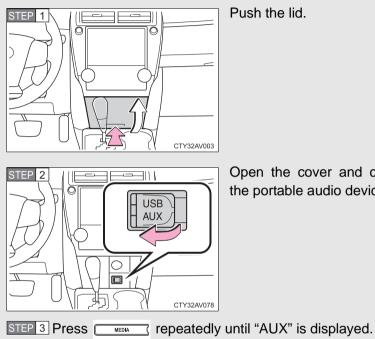
Open the cover and connect the portable audio device.
