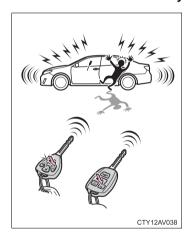
When ((1) is pressed for longer than about one second, an alarm will sound intermittently and the vehicle lights will flash to deter any person from trying to break into or damage your vehicle.
