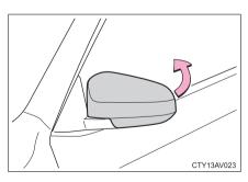
Push the mirror back in the direction of the vehicle's rear.
