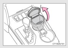
An ashtray can be installed in the cup holder.  $(\rightarrow P. 294)$
