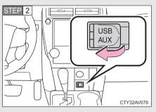
Open the cover and connect an iPod using an iPod cable.
