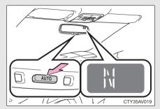
To turn the compass on or off, press "AUTO" for more than 3 seconds.
