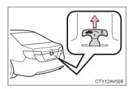
The trunk lid can be opened by pulling up the glow-in-the-dark lever located on the inside of the trunk lid.
