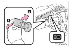
■ With the headlights on, push the lever away from you to turn on the high beams.
