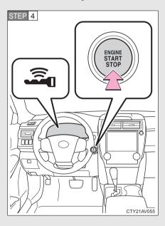
Press the "ENGINE START STOP" switch.
