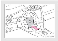
To sound the horn, press on or close to the mark.
