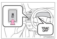
Quickly push and release the switch to turn off TRAC.
