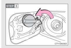
Hang the fuel tank cap on the back of the fuel filler door.
