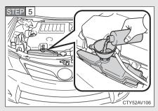
Add engine coolant if necessary.
