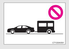
Your vehicle is not designed to be dinghy towed (with 4 wheels on the ground) behind a motor home.
