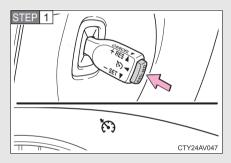
Press the "ON-OFF" button to activate the cruise control.
