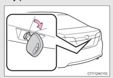
Turn the master key clockwise to release the trunk lid.
