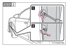
Remove the fender liner clip.
