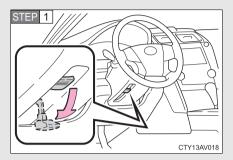
Hold the steering wheel and push the lever down.
