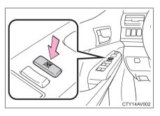
Press the switch down to lock the passenger window switches.
