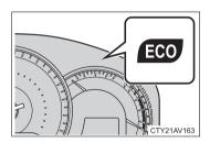
During Eco-friendly acceleration (Eco driving), Eco Driving Indicator Light will turn on. If the acceleration exceeds the Zone of Eco driving, and when the vehicle is stopped, the light turns off.
