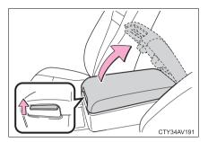
Lift the lid while pulling up the lever to release the lock.
