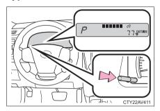
Pressing the button will adjust brightness of the instrument panel lights.
