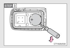
Remove the depleted battery using a small flathead screw-driver.
