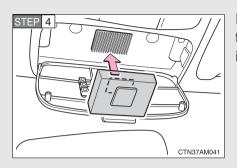
Place the transmitter with the fastener facing inside of box into the box.
