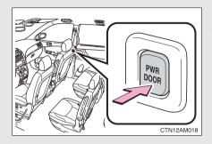
Push the switch to open and close each sliding door.
