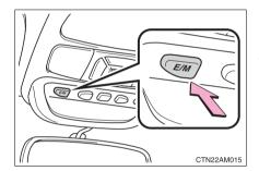
Each time you push the "E/M" button, the display switches (as shown in the following table).
