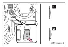
Turn the main switch off to disable the power sliding door system.
