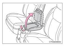
Pull up the knob to release the lock and lift the lid.
