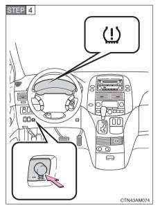
Push and hold the tire pressure warning reset switch until the tire pressure warning light blinks slowly three times.
