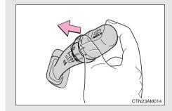
Washer/wiper dual operation Wipers operate automatically.
