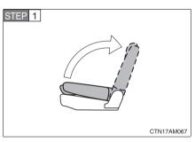
Fold down the seatback by pressing the folding/returning switch ( $\rightarrow$ P. 72). Raise the seatback by pressing the same switch, the returning switch ( $\rightarrow$ P. 76) or the seatback angle adjustment switch ( $\rightarrow$ P. 61). (The seatback will automatically stop.) Do not touch the switch while the seatback is moving, because the operation will stop.
