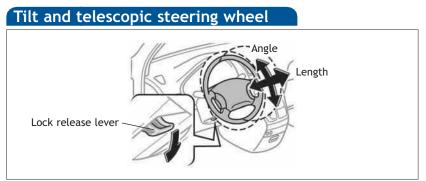
Hold wheel, push lever down, set angle and length, and return lever.
