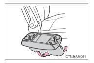
Pull up the lever and push against the driver's seat side.
