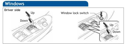
Automatic operation (driver side only) (If equipped) Push the switch completely down or pull it completely up and release to fully open or close. To stop window midway, lightly push the switch in the opposite direction.
