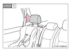
Secure the child restraint using the seat belt or LATCH anchors. Remove the head restraint.
