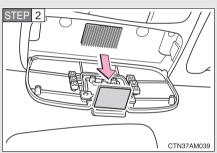
Remove the hook-and-loop fastener.
