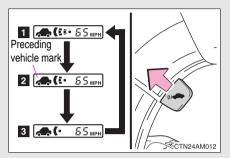
Each pull of the switch toward you changes the vehicle-to-vehicle distance.
