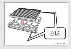
Install a new filter to the filter case.
