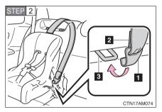
Latch the hook onto the anchor bracket and tighten the top tether strap.
