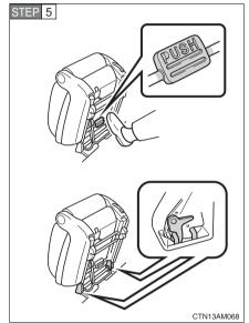
Push the foot pedal forward to securely latch the front leg locks.
