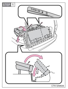
Pull and hold the "TO STOW/ USE" strap and lift up the seat rearward. Then push the seat down.
