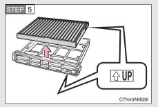
Remove the filter from the filter case.
