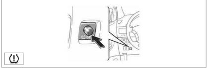
After adjusting tire pressures, or after tires have been rotated or replaced, turn the ignition switch to "ON" and press and hold the "  $\hookrightarrow$  SET" button until indicator blinks three times. Let the vehicle sit for a few minutes to allow initialization to complete.
