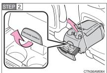
Pull up the lever to disengage the rear lock. Then lift the console box and release the front hook.
