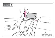
Secure the child restraint using the seat belt or LATCH anchors. Remove and safely stow the head restraint.
