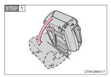
Pull and hold the front leg release strap and fold down the seat.
