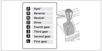
\* The engine switch must be "ON" and the brake pedal depressed to shift from Park.
