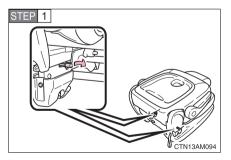
Outer seats: Disengage the rear leg locks by pushing the pins (red) inside each rear leg.
