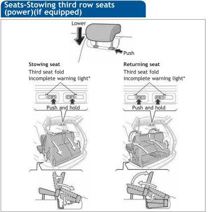
\* This light will remain ON until the seat is fully open or stowed.
