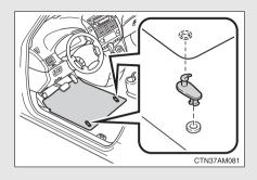
Secure the driver's floor mat using the hooks provided.
