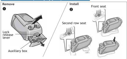
The console box can be removed and installed between the front or second row seats.
