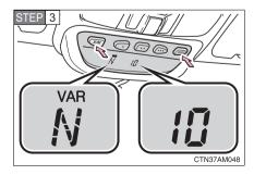
Press and hold both the "MODE" and "E/M" buttons simultaneously for 5 seconds until the "VAR" indication and a number (1 to 15) appears on the compass display. STEP 4 Press the "E/M" button, and referring to the map above, select the number of the zone where you are.
