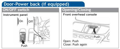
**NOTE:** If battery is disconnected, the power back door needs to be reinitialized. Refer to the *Owner's Manual* for more details.
