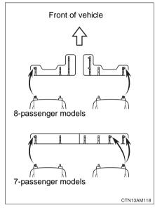
You can distinguish the original seat position by the position of the front leg pins and the shape of the seat striker bezels in the floor.
