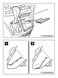
Pull out the partition and place it in the desired position as following illustration.
