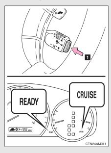
Selecting vehicle-to-vehicle distance control mode
