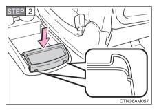
To install the tray (the tray is stored in the console box), hook it onto the outer edge of the console box installation base, then push down on the opposite end to secure it.
