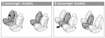
**7-passenger models** The right seat can be placed in the inside or outboard position.
