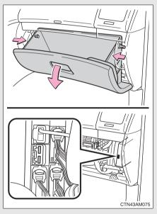
1. Open the glove box. Slide off the damper.
