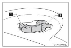
Pull tab **1** out and pull the belt out a little. Then pull tab **2** out.
