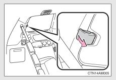
Pull the handle and swing the window fully out to open.
