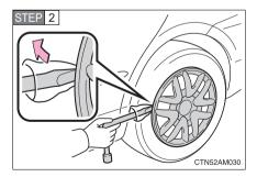
Vehicles with a steel wheel, remove the wheel ornament using the wheel nut wrench.
