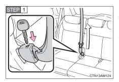
Insert the key into the hole on the center seat belt buckle to release the tab (with the hooked end), and allow the belt to retract.
