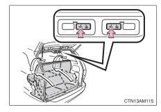
Push and hold the returning switch until the seat cushion is locked.
