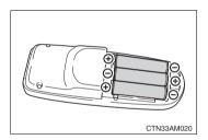
Remove the depleted batteries and install new 3 AA batteries.
