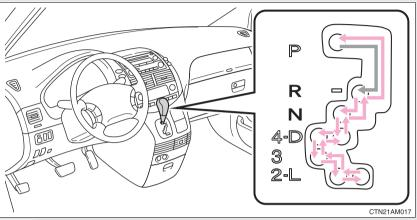
While the engine switch is in the "ON" position, depress the brake pedal and move the shift lever.
