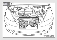
After the engine has cooled down sufficiently, check the engine coolant level and inspect the radiator core (radiator) for any leaks.
