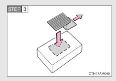
Remove the paper strip covering the adhesive on backside of loop and adhere loop to back side of the transmitter near its center.
