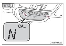
Press and hold both the "MODE" and "E/M" buttons simultaneously for 10 seconds until the "CAL" indication appears on the compass display. (At this time, the compass display is locked in "N".)
