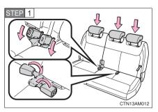
Lower the head restraints to the lowest position and stow the seat belt buckles.
