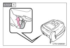
Center seat: Disengage the rear leg locks by pulling the rear leg release lever.
