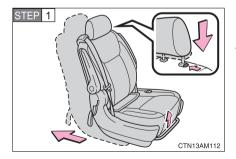
Lower the head restraints to the lowest position and slide the seat to the rear-most lock position.
