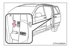
The sliding door cannot be opened from inside the vehicle when the child-protector lock is set.
