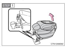
Align the front leg hooks with the rear strikers, then swing up the seat.
