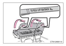
Pull the "TO FOLD/LIFT SEAT-BACK" strap and raise the seatback.
