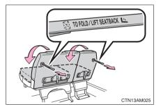
Pull the "TO FOLD/LIFT SEAT-BACK" strap and fold down the seatback.
