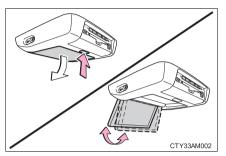
Press the lock release button to open the display.
