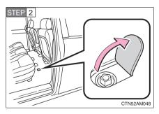
Open the right side sliding door and you will find the flap on the floor. Pull back the flap to find the spare tire clamp bolt.
