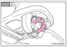
The mirror can be adjusted by pushing its edge.
