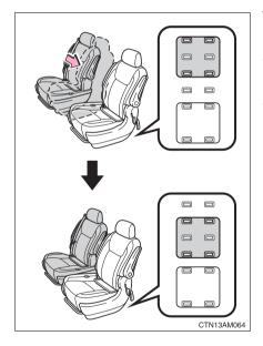
The right side second seat can be moved to the inside when the console box (if equipped) is not installed between the second seats.
