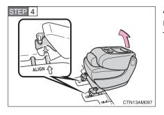
Align the front leg hooks with the rear strikers of the foremost pair. Then swing up the seat.
