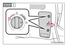
Turn the knobs to the "OPEN" position and remove the cover.
