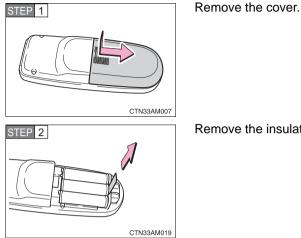
Remove the insulating sheet.
