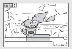
Add engine coolant if necessary.
