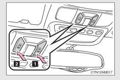
Push and hold the switch to open and close the following door.
