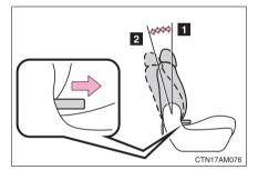
Fold the seatback while pulling the lever. Return the seatback and secure it at the 1st lock position (most upright position). Adjust the seatback to the 5th lock position. ( $\rightarrow$ P. 59)
