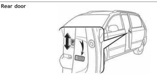
Moving the lever to "LOCK" will allow the door to be opened only from the outside.
