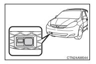
Always keep the sensor clean to ensure that the vehicle-to-vehicle distance control operates properly. (Some obstructions, such as snow, ice or plastic objects, cannot be detected by the obstruction sensor.)
