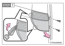
Remove the securing bolts and remove the unit.
