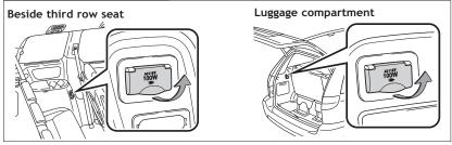
Designed for car accessories. Engine switch must be in the "ACC" or "ON" position to be used.
