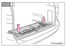
Push the seat against the floor and make sure it is locked securely.
