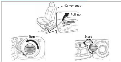
**NOTE:** Tighten until one click is heard. If the cap is not tightened enough, Check Engine " $\bigoplus_{m \in K}$ " indicator may illuminate.
