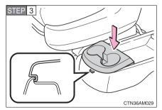
To install the cup holder, hook it onto the outer edge of the console box installation base, then push down on the opposite end to secure it.
