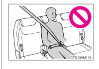
Do not use the center third seat belt with either buckle released. Fastening only one of the buckles may result in death or serious injury in case of sudden braking or a collision.
