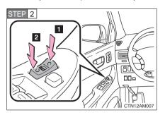
Shift the shift lever to P or N, and press and hold the driver's door lock switch ( or 2) for approximately 5 seconds and then release.
