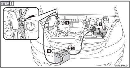
Connecting the jumper cables
