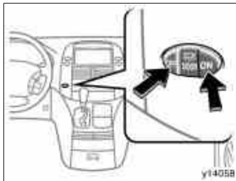
Personal light main switch
