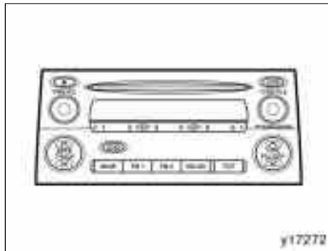
Type 2-1: AM-FM radio/compact disc player with changer (with XM® satellite radio* controller)
