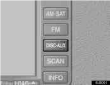
(c) Playing a disc Push the “DISC-AUX” button if a disc is already loaded in the player. “DVD” appears on the screen. (If the CD changer is turned on, push the “DISC” button again to switch to the DVD player.)
