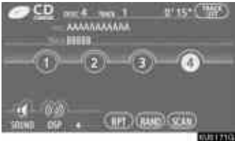
(d) Selecting a desired disc Touch the desired disc number on the screen. The changer will start playing the selected disc from the first track.
