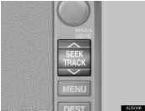
SELECTING A DESIRED TRACK “SEEK/TRACK” button: Use for direct access to a desired track. Push either side of the “SEEK/TRACK” button and repeat it until the desired track number appears on the display. As you release the button, the player will start playing the selected track from the beginning. “TRACK LIST”: The desired track can be selected from a list. This function is available only when the vehicle is not moving. Touch “TRACK LIST”. The track list is displayed.
