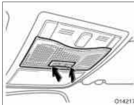
Interior light switch
