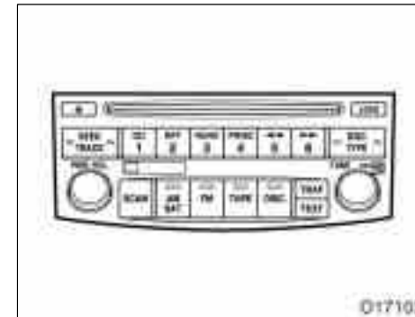
Type 3: AM-FM radio/compact disc player with changer (with cassette player and XM® satellite radio* controller)
