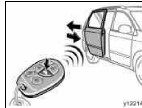
Right side power sliding door (type B)
